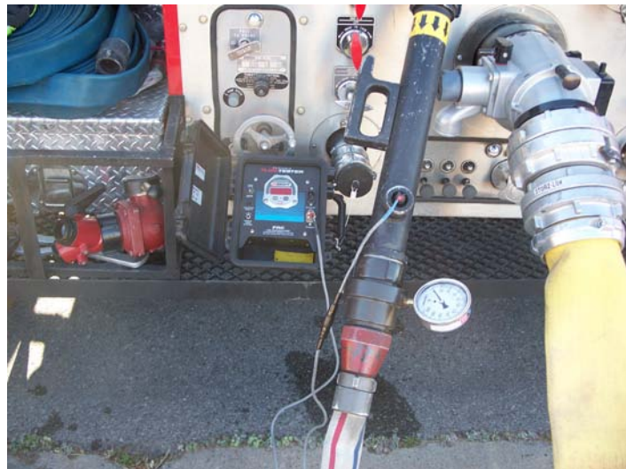
An assortment of gauges as well as a flow meter assured test accuracy
